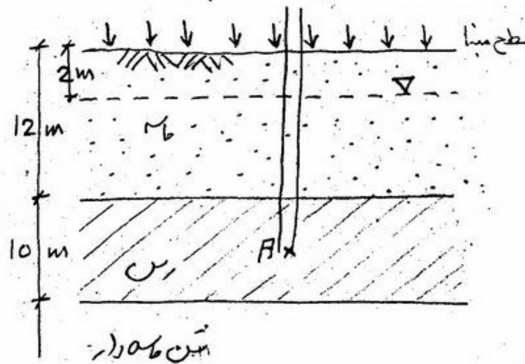
$$\text{Water Head} = \frac{\Delta P}{\gamma} = \frac{200}{10} = 20 \text{ m}$$
