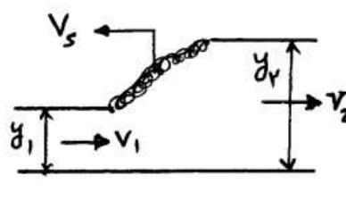
$$V_1 y_1 = V_2 y_2 \quad (1)$$
