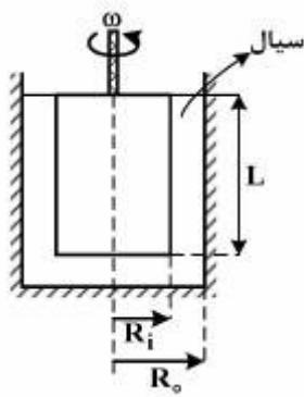
$$\frac{R_i^\tau \mu \omega}{R_o - R_i} \quad (1)$$
