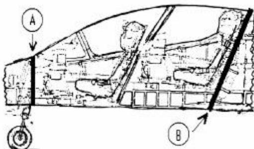
A: Aft Pressure Spar و A:Front Pressure Spar (۱)
