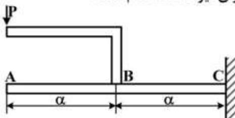
$$V(x) = -p(x-a)^1 \quad M(x) = -\frac{p}{2}(x-a)^2 - pa(x-a)^0 \quad (1)$$
