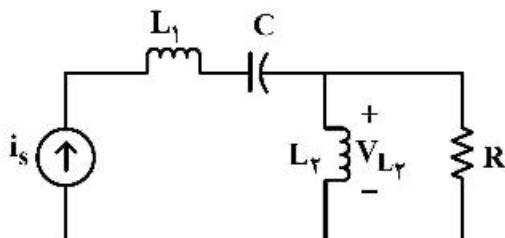
$$V_{L_2}(t) = R\delta(t) - \frac{R}{L_2} e^{\frac{-Rt}{L_2}} u(t) \quad (1)$$
